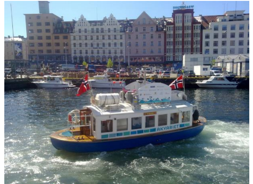
H2 fueled 12,5 kW FC system incl batteries and electric propulsion installed on MF Vågen (2009-2011)
