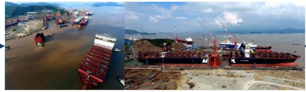
Floating in & out vessel new and existing sections
